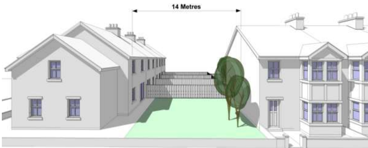
Figure 3 Principal window and two storey secondary elevation
