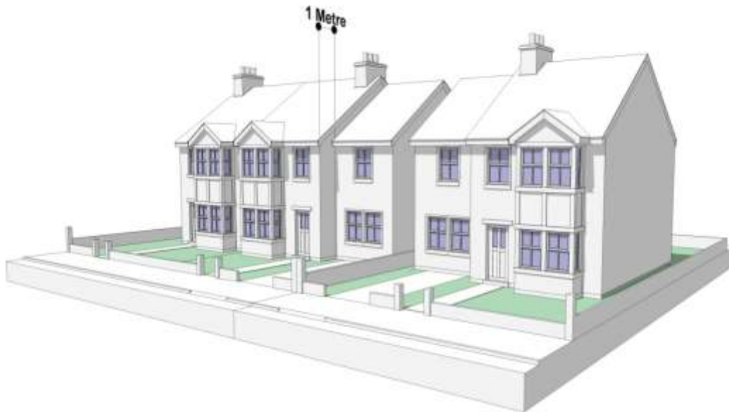
Figure 9 One Metre Gap to the Side Boundary
