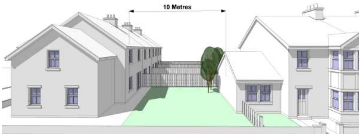
Figure 4 Principal window and single storey secondary elevation
